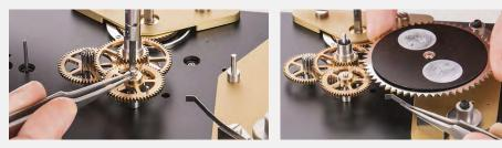
When putting on the moon disc wheel, please ensure that the driving pin of the moon driving wheel is exposed and is not jammed by the moon disc wheel.
