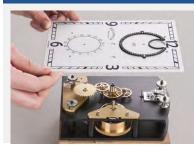
Carefully place the pre-assembled dial on the four knurled nuts of the pillars\* and secure them using four cylinder-head screws M2 x 4.
