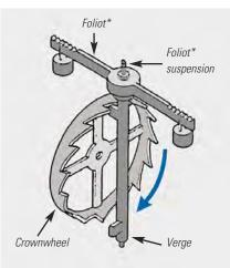
of rotation until the escapement reached its inversion point\* after dropping the Verge escapement pallet (later the escape wheel tooth). The escapement was thus attached to the gear train\* during the entire duration of its oscillation.
