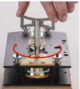
So that your timepiece can be wound via the mainspring in the spring barrel (red arrow), the click allows it to only move in one direction (blue arrow).
