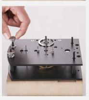
After screwing the plates<sup>\*</sup> examine the endshake of the arbors<sup>\*</sup> in order to avoid the bearings sticking. To do this, carefully grasp the arbors with the tweezers and move them toward the pivots. If you turn the movement over, you should be able to acoustically hear the arbors fall onto the bearings.
