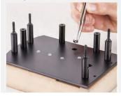
Another change to the standard movement is the positioning of the large spring barrel ball bearing. Like the protective pillars, this is inserted into the ball bearing pocket on the righthand side of the back plate. As a result, the lowest ball bearing pocket of the back plate remains empty here as well.
