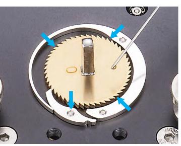
Only use the oil made especially for clocks delivered with this clock kit in the syringe - Möbius Microgliss D5 - and follow directions on how to properly lubricate in the section »Using the Tools« on page 19 of this booklet
