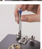
The escapement can now be carefully screwed to the front plate using two cylinder-head screws M2 x 4.
