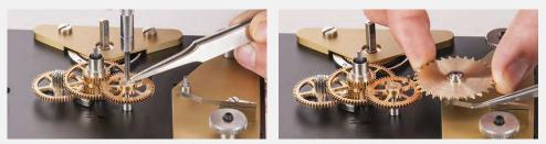
When putting on the date wheel, please ensure that the driving pin of the date driving wheel is exposed and is not jammed by the date wheel.
