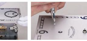
Carefully place the pre-assembled dial on the four knurled nuts of the pillars  $^*$  and secure them using four cylinder-head screws M2 x 4.
