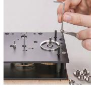
The three protective pillars are screwed in using M4 x 10 countersunk-head screws. Screwing this is very important to avoid accidental opening of the movement!
