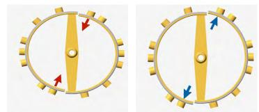
When heated, the outer layer expands more strongly, thus pushing the inner layer toward the center of the balance. This change in inertia accelerates the balance wheel and compensates for the softer balance spring when heated. When cooled, the outer layer consolidates more strongly. The diameter of the balance wheel increases and the balance gets slower. The increased inertia of the balance wheel is thus the same as the cooling of the increasingly strong and hard balance spring.
