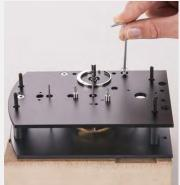
The three protective pillars are screwed in using M4 x 10 countersunk-head screws. Screwing this is very important to avoid accidental opening of the movement!
