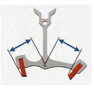
The following illustrations show the most important phases of the interplay between the escape wheel\*, pallet\* lever, and balance\*.
