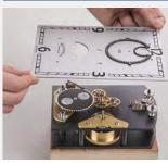
Carefully place the pre-assembled dial on the four knurled nuts of the pillars\* and secure them using four cylinderhead screws M2 x 4.
