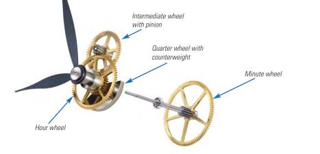
Out of all these points a solid gear train is created that meets the standards of a table clock in every way.
