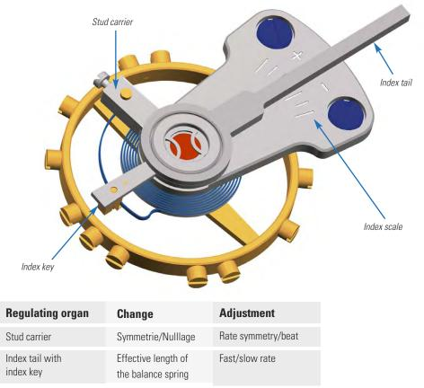
Changing the effective length of the balance spring\* during regulation with the index system (guiding the balance spring using the index tail) by only a tenth of a millimeter already leads to a rate change of more than one second per day
