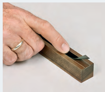
Fitting the seal to protect the movement from dust
