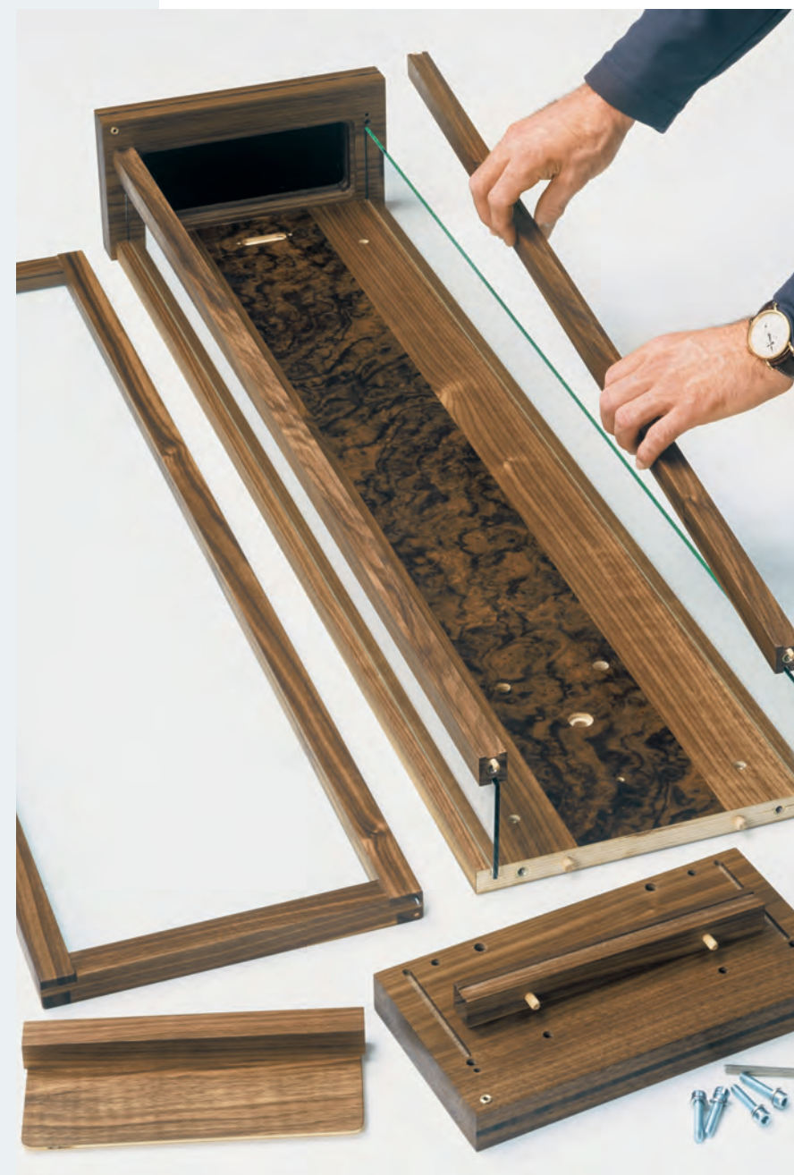
Fitting the seal to protect the movement from dust
