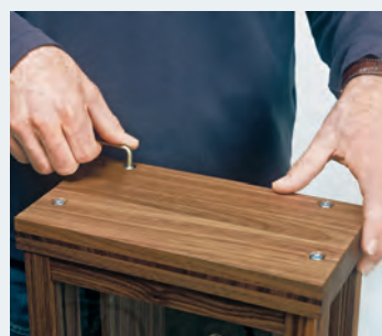
Easy assembly of the case parts with Allen screws
