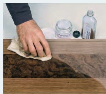
Surface treatment of the natural wood case with care oil based on natural ingredients
